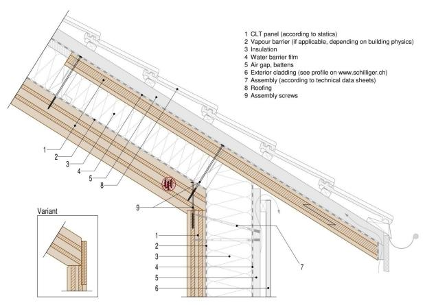
This detail can be applied to single-storey or multi-storey wooden buildings. It serves as an aid and does not replace a building concept. The detail must be adapted according on static, building physics and fire safety requirements. Variants with different products are possible. Our technical office is at your disposal for any questions you may have.
